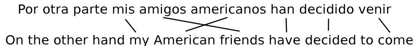
Figure 1: Example of word alignment obtained by tracing back the operations done by Apertium when translating from Spanish to English the sentence Por otra parte mis amigos americanos han decidido venir . Note that por otra parte is analysed by Apertium as a multi-word expression whose words are left unaligned for convenience (see section 4.2).
