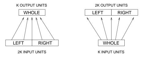
**Figure 2.** *Proposed feedforward networks for the Compressor and Reconstructor working with binary trees.*
